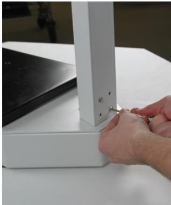
Figure 2-3. Attach Eight Bolts and Washers to Secure the Pillar to the Scale Base
