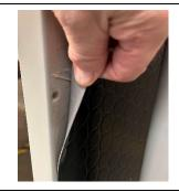
14. With the utility knife or scissors cut a small v shape around the 2 holes to make them accessible.
