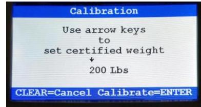
8. The display will prompt for the calibration weights to be placed on the platform. Press **Enter** after calibration weights are placed on the platform.
