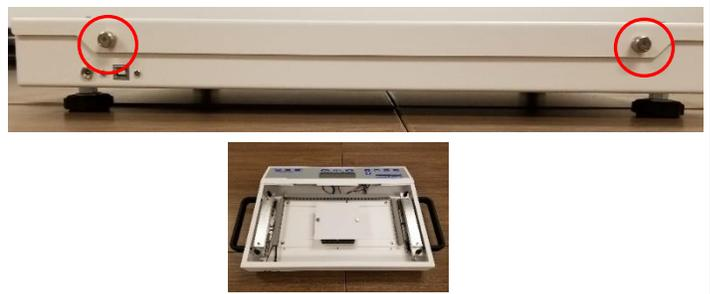
2. If batteries are installed, remove the two thumb screws on the top of the battery compartment located in the center of the inside of the scale and remove the batteries. Set aside to reinstall in step 3. If batteries are not installed, skip to the next step.
