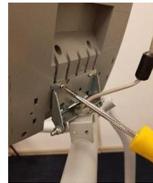
4. Use the Phillips head screwdriver to remove the 6 screws on the rear of the display head. Carefully open the display head, ensuring not to damage internal components. Do not touch any circuitry, ribbons or cables other than the keypad ribbon. Tape may be loosened or temporarily removed to allow the display head to be opened more easily.
