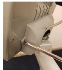
3. Use the Phillips head screwdriver to remove the display head from the mounting bracket on the top of the scale.
