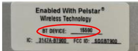
**SERIAL NUMBER AND BT DEVICE NUMBER MUST MATCH TO ENABLE WIRELESS COMMUNICATION**
