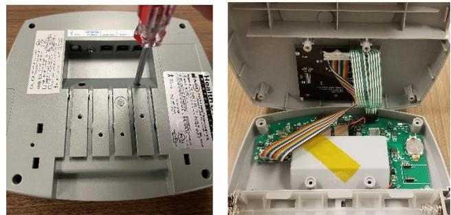
5. Carefully insert the wireless module into the 8 pin socket located on the green PC board as shown. Observe the orientation of the wireless module as shown. Gently press until secure, do not apply extreme pressure.
