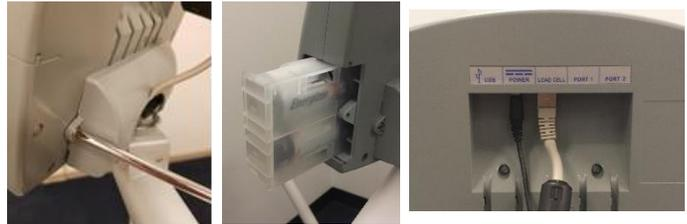
2. Use a Phillips head screwdriver to remove the display head bracket cover on the back of the display head.
