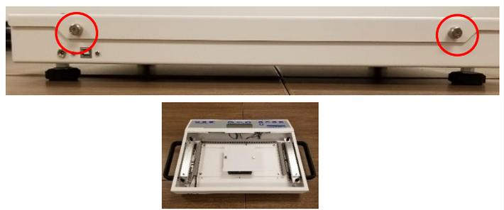
2. If batteries are installed, remove the two thumb screws on the top of the battery compartment located in the center of the inside of the scale and remove the batteries. Set aside to reinstall in step 3. If batteries are not installed, skip to the next step.
