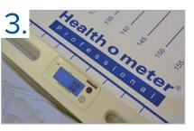
Lay the Patient Transfer scale flat onto the stretcher or bed and turn the scale on by pressing the blue power button.
