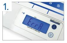
While preparing to weigh a patient, ensure there are no more than 8" between each stretcher/bed or stretcher/ stretcher. The scale should not be tilted and must be as level as possible. The PTS has an electronic level and if the scale is not flat an "ERR A" message will appear. If the "ERR A" code does appear, do not remove the patient from the scale, just lower one surface until level and the weight comes up.
