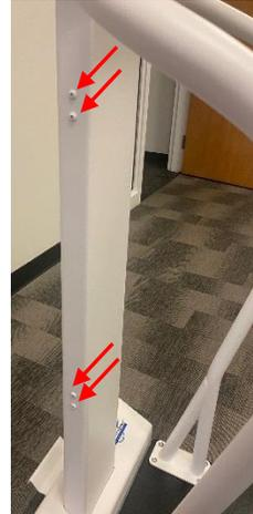
2. Position the height rod with mounting brackets onto the scale as shown. Use the screws removed in step 1 to attach the height rod to the scale. DO NOT FULLY TIGHTEN THE SCREWS AT THIS TIME.
