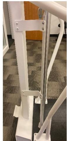
3. Ensure that the height rod is positioned with the red locating fixture seated on the top surface of the black scale platform. Fully tighten all four screws on the scale pillar.
