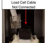
2. Inspect the load cell connector cable to ensure it is completely plugged into the RJ jack. If cable was plugged in, unplug and plug in again until it clicks into place. After checking connection, replace door at the back of the platform base or reassemble the platform and column.
