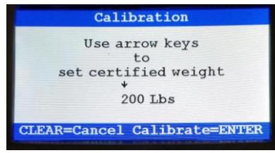
9. The display will prompt for the calibration weights to be placed on the platform. Press **Enter** after calibration weights are placed on the platform.
