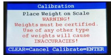
10. The display will show "Calibrating" during the calibration process.
