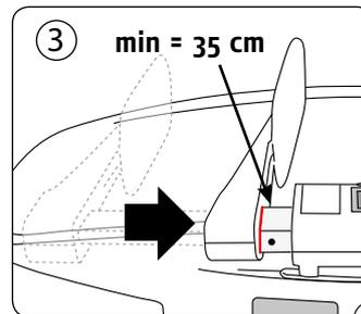
Slide the measuring panel all the way in towards the digital display.
