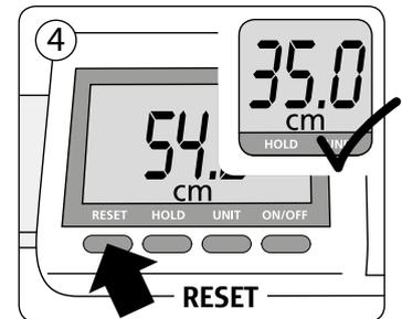
Press **RESET** to set the height reference point at 35 cm. This step must be done each time the height rod is powered on.
