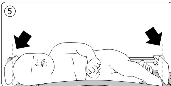
Place the baby on a flat surface. Position the non-moving panel at the baby's head. Stretch the baby's legs and slide the measuring panel towards the baby's feet.
