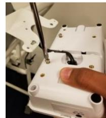
8. Align the display head with the mounting bracket located on the handrail. Attach the display head to the mounting bracket by inserting the two screws removed in the previous step through the bracket and into the display head.
