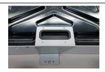
3. Obtain the four self-drilling screws from the packaging. Using a power drill, insert the four screws through the holes in the bracket into the underside of the scale.
