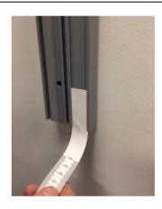
9. To position the measuring tape at the correct height, place the zero of the measuring tape flush with the floor. Ensure that the zero is at the floor, not the end of the tape.
