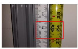
11. Once positioned at the correct height, obtain one of the measuring tape retaining clips from the bag. Secure the measuring tape to the height rod channel by attaching the clip at the bottom of the height rod channel.
