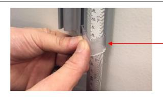
12. Obtain the headpiece from the carton. Align the grooves at the back of the headpiece with the grooves at the top of the height rod. Gently lower the headpiece onto the height rod. The tension knob may need to be loosened to allow the headpiece to slide onto the height rod channel.
