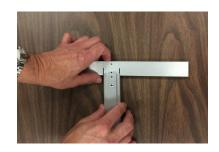
Insert the two 1/2" screws from the clear bag into the holes at the bottom of the height rod. Use a Phillips head screwdriver to tighten the screws securely.
