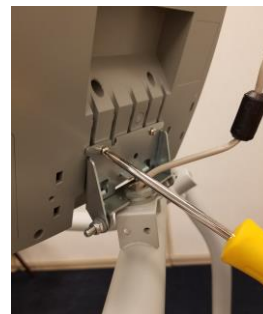
Slide slots onto tabs in bracket
