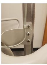
6. Position Height Rod in front of the Upper and Lower HR Mount Brackets so that the 2 holes in the Lower HR Mount Bracket are positioned over the 2 threaded holes on the back of the HR assembly. Thread 2 each ½"-20 x 5/16" Button Head Screws into the threaded holes on the rear of the Height Rod Assembly. Tighten both Screws with 5/32" Wrench.
