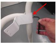
3. Using the provided 8mm Allen Wrench, remove and discard the M10 x 1.5 x 40mm Socket Head Screw from the bottom of the Left Handrail.
