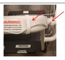
10. Secure the height rod cable and load cell cable into the display head bracket cover as shown. Plug the cable from the height rod into Port 2. Assembly is complete. If experiencing connection issues, contact Health o meter® Professional Scales Technical Support at 1-800-638-3722
