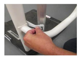
7. To ensure height accuracy the height rod must be level with the platform. Obtain the included leveling guide\* and slide onto the left top portion of the platform. The black cap on the bottom of the height rod should lie flush on top of the guide. If adjustment is needed, loosen the button head screws in the mounting brackets and adjust until flush. \*leveling guide may be red or gray
