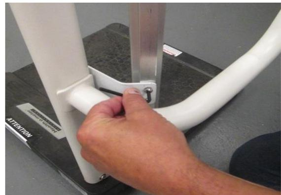
7. To ensure height accuracy the height rod must be level with the platform. Obtain the included leveling guide\* and slide onto the left top portion of the platform. The black cap on the bottom of the height rod should lie flush on top of the guide. If adjustment is needed, loosen the button head screws in the mounting brackets and adjust until flush.
