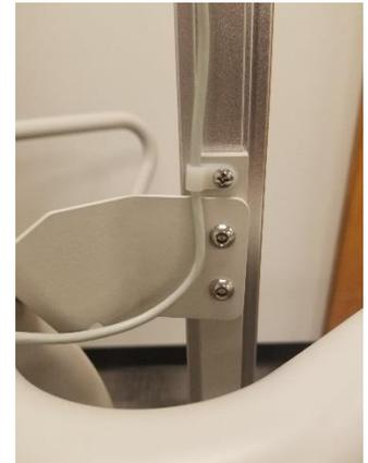
6. Position Height Rod in front of the Upper and Lower HR Mount Brackets so that the 2 holes in the Lower HR Mount Bracket are positioned over the 2 threaded holes on the back of the HR assembly. Thread 2 each 1/4"-20 x 5/16" Button Head Screws into the threaded holes on the rear of the Height Rod Assembly. Tighten both Screws with 5/32" Wrench.
