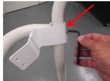
3. Using the provided 8mm Allen Wrench, remove and discard the M10 x 1.5 x 40mm Socket Head Screw from the bottom of the Left Handrail.
