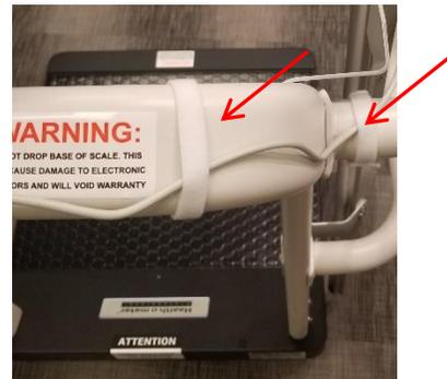
10. Secure the height rod cable and load cell cable into the display head bracket cover as shown. Plug the cable from the height rod into Port 2. Assembly is complete. If experiencing connection issues, contact Health o meter® Professional Scales Technical Support at 1-800-638-3722
