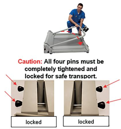
3a. Using the handles on the end of the platform, carefully lift the scale vertically onto its base where the wheels are located.
